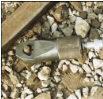
◀ Easily removing rusty nuts during railroad construction is just one of many application examples for the Enerpac Nut Splitter.
