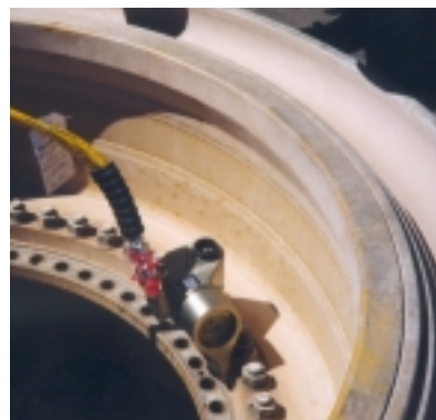
An Enerpac hydraulic torque wrench brings safety and economy, along with reliable maintenance and reduces operator fatigue.
