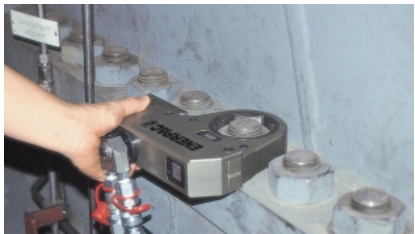
The hexagon cassette hydraulic torque wrench. The slim nose radius and swivel couplers allow easy access in all positions.
